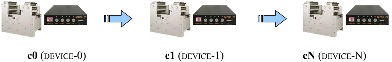
Connecting an EMUFDD “on-the-fly” it's very easy. You only need to modify, on each machinery, the floppy flat and power supply cables with longer ones, coming out from the machinery/control. After this modify, connecting/disconnecting the EMUFDD will be as easy as connecting/disconnecting a USB key and fast, since there's no more need to open the machinery to reach the floppy cables.
