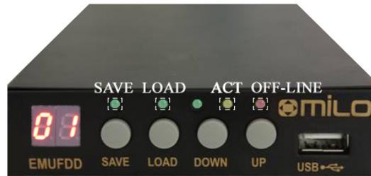
EMUFDD configuration is plug'n'play and absolutely jumper-free. It's also possible to configure the emulator with up to 100 different configurations and switch, at run-time, between them. The first 10 configurations (c0÷c9) can be loaded with any custom setting, the other 90 configurations (0.0÷9.0) are fixed presets.
