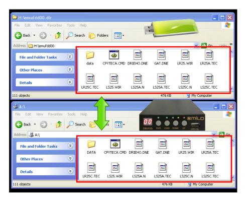
[top window]USB key (H:) in the PC server[bottom window]EMUFDD (A:) in the machinery
